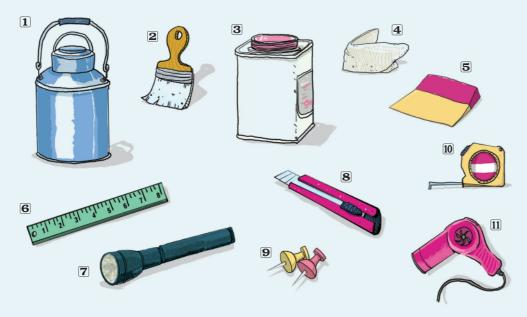
1 Primer (PM02, PM04) 2 Brush 3 Cleaning solvent (alcohol, white gasoline or lacquer thinner) 4 Lint 5 Plastic applicator 6 Steel ruler 7 Torch 8 Stanley knife (45° angle) 9 Needle or pin 10 Measuring tape 11 Hair dryer 12 Other: sandpaper, putty stick, sealer, masking tape, gloves
