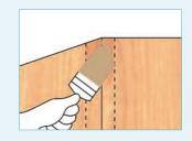
When LG Hausys Interior Film is applied to internal corners, firstly apply primer to the corner covering at least 50mm of each surface. This will ensure maximum adhesion.
